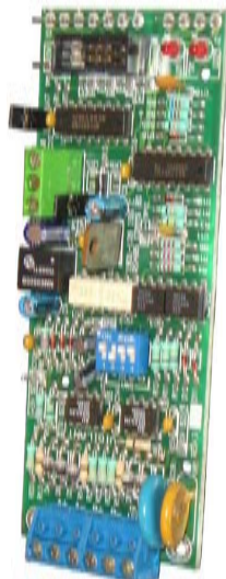
PA0711 RS485 Comms PCB 1901-139-1 Plug-on (Modem connection to F4000 Main Board - external power)
