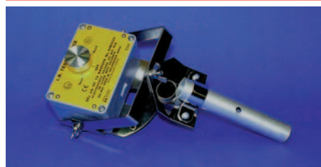
Part Number 592.001.012 T110 Test Source for use with SOLO 704 Adaptor Tube B and SOLO100/101 poles
