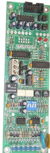
PA0712 RS485 to RS232 PCB 1901-139-2 (RS232 to RS485 - external power)
