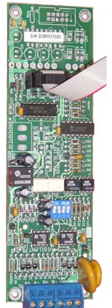
PA0773 RS485 Comms CMOS PCB 1901-139-3 FRC Only (FRC connection - including power)
